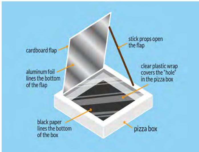
step that we took was to get some tin foil wrap and cut two pieces the size of the pizza box and tape them to the inner top and bottom of the pizza box and cut out tin foil pieces for the inner sides of the box. Tape all
