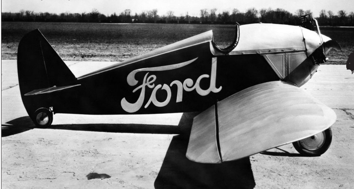
Ford Flivver, about 1927, with full-span ailerons. Source: San Diego Air and Space Museum Archives.
